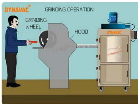
Dust extraction through exhaust hood fitted around grinding wheel
