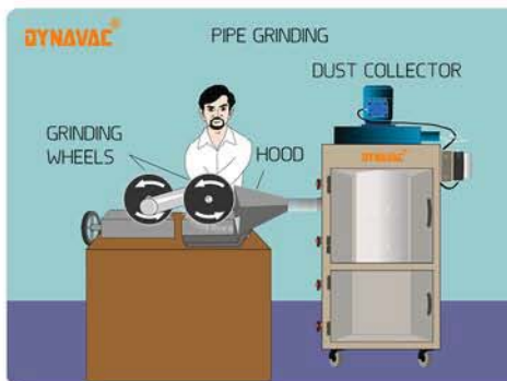
Dust extraction from pipe grinding operation
