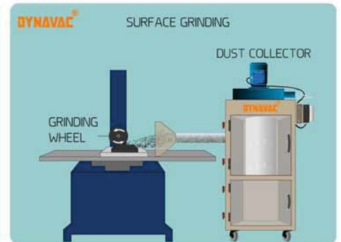
Dust collection from surface grinding operation
