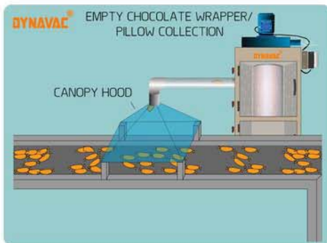
Empty wrappers collection on a conveyor belt with adjustable canopy hood
